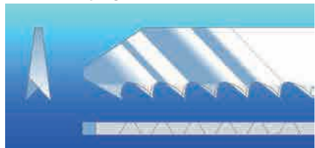
Ground and taper ground teeth
